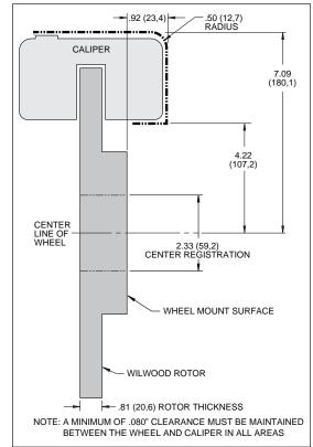
Figure 2. Wheel Clearance Diagram
